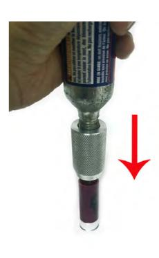
Push the charger downward by force to charge. Charge for 3 – 5 sec to fill up the cartridge shell
